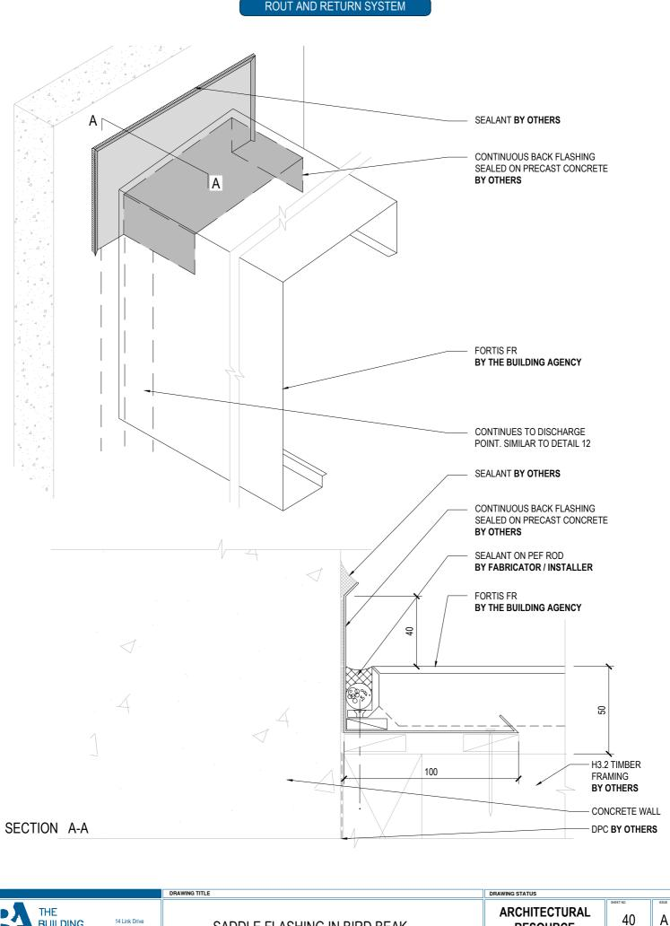
SADDLE FLASHING IN BIRD BEAK RESOURCE SCALE @ A4: 1:2 DATE: March 2025 Copyright © of this drawing shall remain the property of The Building Agency. No part of this document may be reproduced or transmitted by any m
