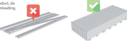
• INNOWOOD material should be stored undercover and protected from the elements (including direct sunlight and rain) until ready to install. Remove any plastic wrap including shrink wrap and store on a dry and flat surface supported at a maximum 450mm centres.
