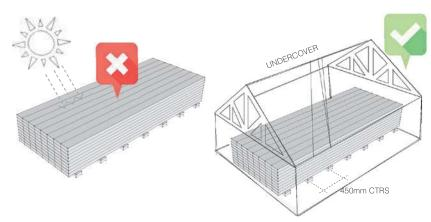
INNOWOOD material should not be stored in the open or covered or wrapped with plastic. Use a breathable membrane to cover the boards.
